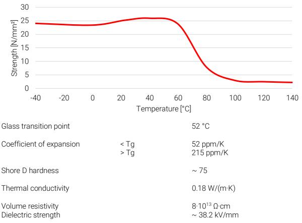
Tensile shear strength acc. to DIN EN 1465
